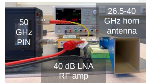
Radio-over-fiber (RoF) receiver implementing photonic up-conversion to mmWave (26.5 – 40 GHz) frequencies for 5G applications.
