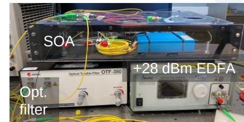
SOA (+16 dBm output) and EDFA (+18 dBm) amplifiers, C-band optical filter with tunable wavelength and bandwidth.
