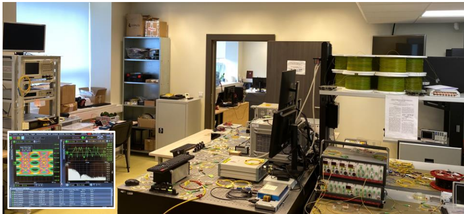
Adaptive fiber optical communication systems testbed for intensity modulated WDM systems being regularly upgraded.
