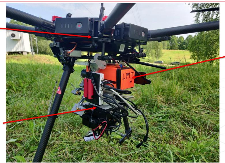
Camera, Wi-Fi router, PC with software
